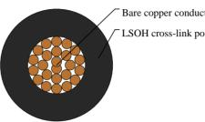
Bare copper conductor LSOH cross-link polyolefin insulation
